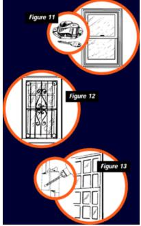
outside sash. The window can then be secured by inserting nails through the holes which prevent it from being raised. (Figure 13)
