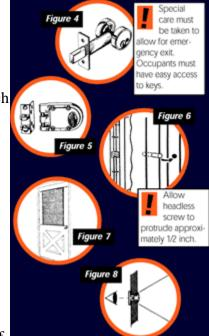
midway between the hinges. Drill an opposing hole in the door jamb to receive the screw when the door is closed. (Figure 6)
